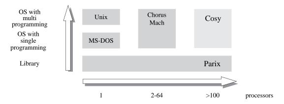
Fig. 1: Cosy in the spectrum of operating systems
