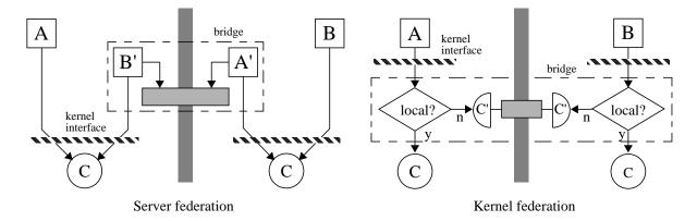
Fig. 2: Communication between processes, in the server federation (left) and in the kernel federation (right).
