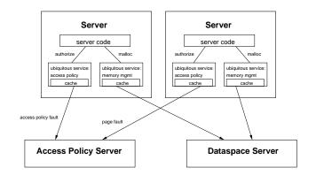
Figure 2: The SawMill approach enables the decomposition of monolithic operating systems into individual system servers where ubiquitous services manage server data obtained from resource servers locally.
