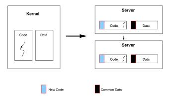
Figure 1: Decomposing a monolithic operating system into a multiserver operating system involves: (1) additional communication between between servers; (2) buffer management for common data in multiple tasks; and (3) the addition of new code to compose a system from independent servers.
