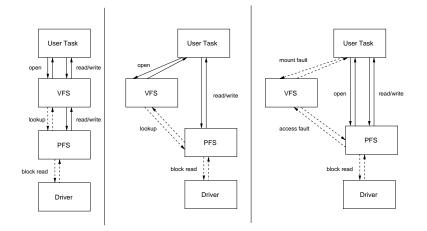
Figure 3: The communication requirements for three file system protocol options. Dashed IPCs are optional. For example, a PFS lookup may not be necessary because the appropriate inodes may be present in the directory cache.
