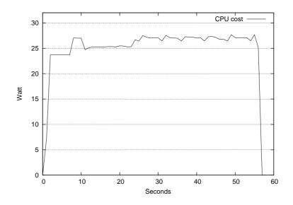
Figure 5.6: Total energy consumption of two simulaneous runs of factor.
