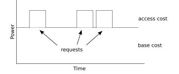
Figure 3.3: Simplified power consumption of a device, split into base cost and access cost.
