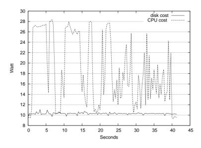
Figure 5.3: Total energy consumption of two simulaneous Postmark runs.
