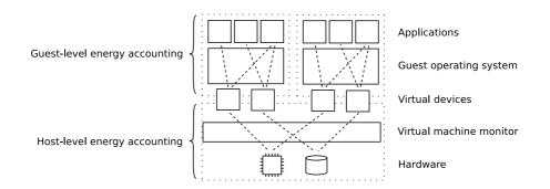
Figure 1.1: Overview of our approach. The virtual machine monitor estimates the energy consumption of the hardware and accounts it to the virtual machines. Each guest operating system obtains the energy consumption of the virtual devices and charges it to the running applications.
