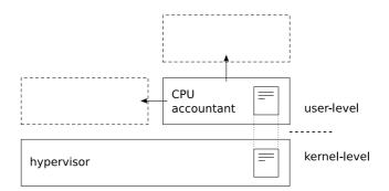
Figure 3.2: User-level accounting of CPU energy consumption. The priviledged hypervisor writes information about the CPU into a log file shared with a user-level CPU accountant. The CPU accountant analyzes the log entries and charges the energy consumption of the CPU to other components (e.g. to user-level device drivers or virtual devices).
