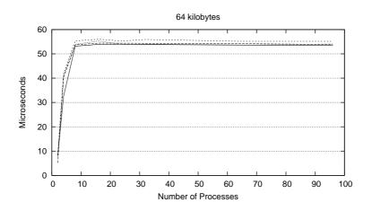
Figure 5.1: Context switch latency measured with lat\_ctx.
