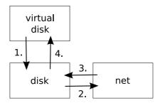
Figure 3.4: Recursive accounting of energy consumption. The virtual disk sends a disk request to the shared disk driver (1.). To fulfill the request, the disk driver uses the network driver (2.), which estimates the cost for processing the request and returns it to the disk driver (3.). Finally, the disk driver charges the energy consumption of the disk and the network interface to the virtual disk (4.).
