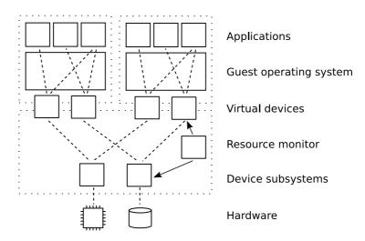
Figure 3.1: Overview of the accounting architecture. Accounting components in each device subsystem estimate the energy consumption of the device and apportion it between the virtual devices. The virtual devices export their energy consumption to the guest operating system, which charges it to its resource principals. Based on the accounting information provided by the device subsystems, the resource monitor controls the energy consumption of physical and virtual devices.
