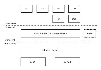
Figure 4.1: Environment: Upon a Pentium D, 2x3GHz, a L4 micro-kernel driven virtualization environment hosts a various number of guest virtual machines.
