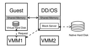
Figure 3.3: DD/OS - Client Architecture
