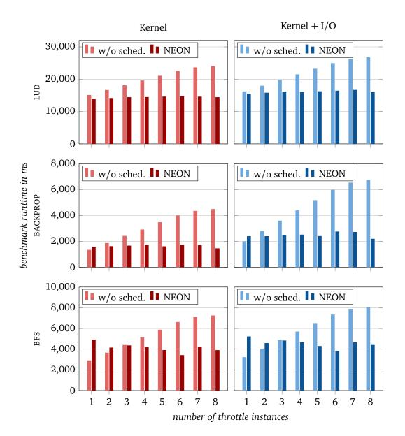
Figure 5.8: Fairness enforcement between a virtual machine and a host task with our paravirtual approach. Shown are the runtimes of the rodinia benchmarks LUD, BACKPROP, and BFS. Each benchmark runs eight times on the host, with increasing numbers of throttle instances in the guest, resulting in longer benchmark runtimes. A perfect scheduler keeps the benchmark runtimes constant, independent of the number of throttle instances in the virtual machine.
