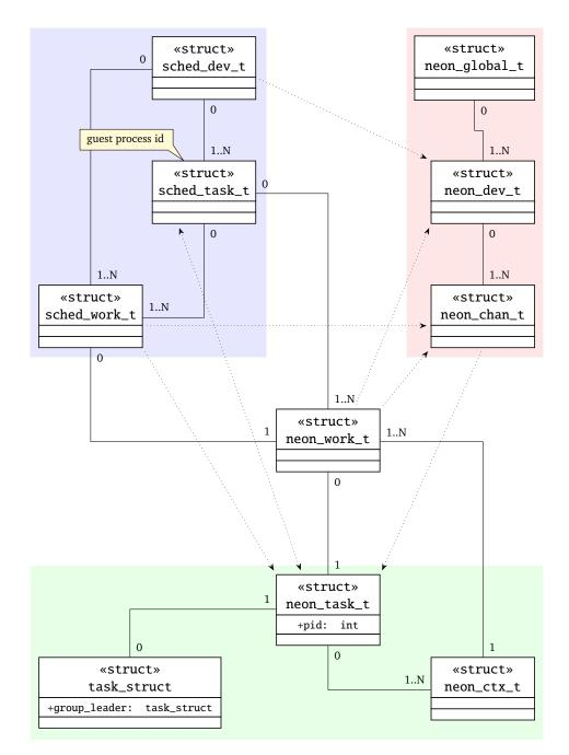
Figure 4.3: NEON's internal data structures. Straight lines denote direct references (pointers), dotted lines denote indirect references via ids. We add the guest process id to neon\_task\_t in order to support grouping. task\_struct is a Linux kernel data structure. The colored groups are explained in Section 4.3.3.
