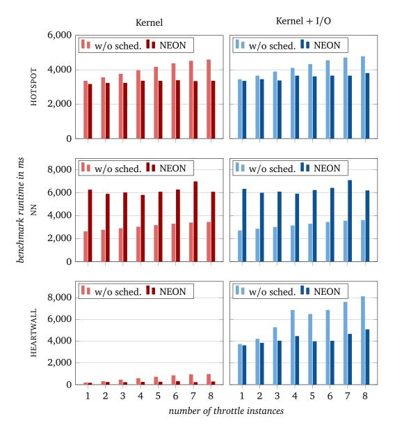
Figure 5.9: Fairness enforcement between a virtual machine and a host task with our paravirtual approach. Shown are the runtimes of the rodinia benchmarks HOTSPOT, NN, and HEARTWALL. Each benchmark runs eight times on the host, with increasing numbers of throttle instances in the guest, resulting in longer benchmark runtimes. A perfect scheduler keeps the benchmark runtimes constant, independent of the number of throttle instances in the virtual machine.
