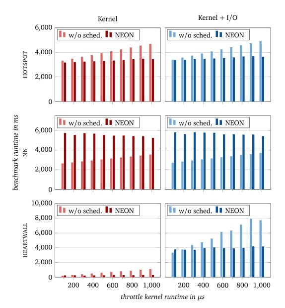
Figure 5.3: Baseline of NEON's scheduling capabilities. Shown are the runtimes of the rodinia benchmarks HOTSPOT, NN, and HEARTWALL. Each benchmark runs ten times alongside the throttle application. We configure throttle to create increasing amounts of load. Without any scheduling, throttle occupies increasingly larger shares of GPU time, resulting in longer benchmark runtimes. A perfect scheduler keeps the benchmark runtimes constant, independent of throttle's kernel runtime.
