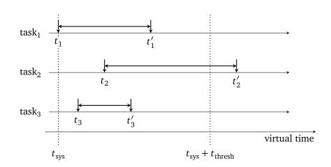
Figure 2.5: Disengaged fair queuing: NEON manages individual GPU time counters for each task and predicts the counter values at the end of an beginning freerun phase by interpolating the GPU utilization measured during sampling. If this prediction exceeds a threshold, the application is not allowed to use the GPU in the upcoming freerun phase.
