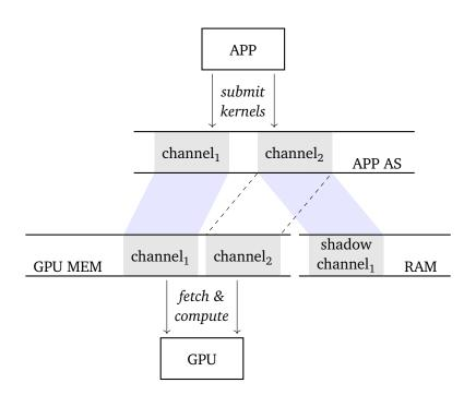
Figure 2.3: Shadow channels: A shadow channel is a transparent modification to an application's channel mapping. Instead of pointing to GPU memory, the shadowed channel points to a kernel buffer in system RAM. When the application submits kernels into a shadowed channel, they do not reach the GPU. Here, channel<sub>1</sub> is active with a regular mapping, channel<sub>2</sub> is shadowed.
