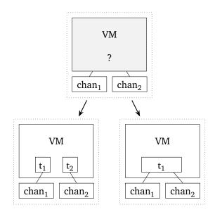
Figure 3.3: Two possible solutions for the observation: "One VM, two channels". There are either two guest tasks, using one channel each, or just one, which uses both channels. Without additional information, NEON cannot distinguish the two.
