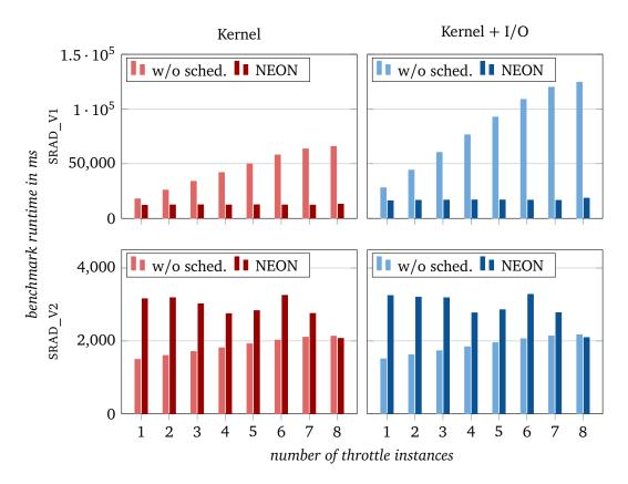
Figure 5.10: Fairness enforcement between a virtual machine and a host task with our paravirtual approach. Shown are the runtimes of the rodinia benchmarks SRAD\_V1 and SRAD\_V2. Each benchmark runs eight times on the host, with increasing numbers of throttle instances in the guest, resulting in longer benchmark runtimes. A perfect scheduler keeps the benchmark runtimes constant, independent of the number of throttle instances in the virtual machine.
