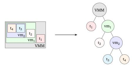
Figure 3.4: Representation of nested virtualization. On each level, the scheduler must divide the available GPU computation time fairly
