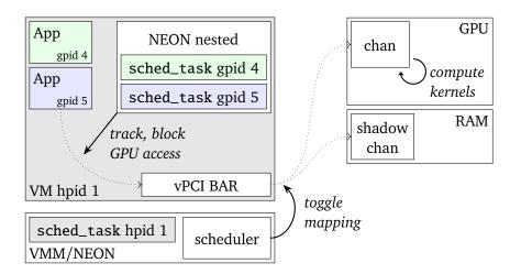
Figure 3.6: Structure of the nested approach: Thy hypervisor accounts and controls the virtual machine as a whole by using shadow channels, similar to the paravirtual approach. Fairness inside the virtual machine is enforced by the nested scheduler, which tracks and controls applications based on their mapping of the virtual PCI BAR device.
