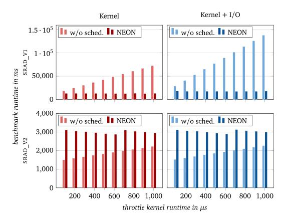
Figure 5.4: Baseline of NEON's scheduling capabilities. Shown are the runtimes of the rodinia benchmarks SRAD\_V1 and SRAD\_V2. Each benchmark runs ten times alongside the throttle application. We configure throttle to create increasing amounts of load. Without any scheduling, throttle occupies increasingly larger shares of GPU time, resulting in longer benchmark runtimes. A perfect scheduler keeps the benchmark runtimes constant, independent of throttle's kernel runtime.
