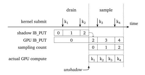
Figure 4.2: Wrong accounting after unshadow: NEON expects channels to be empty before sampling starts. With shadow channels, this is no longer true, because applications can submit kernels while being blocked. The GPU computes four kernels in total: Two, that were submitted into the shadow channel during the draining phase, and two submitted during sampling. This invalidates NEON's accounting, which only sees the later two kernels.
