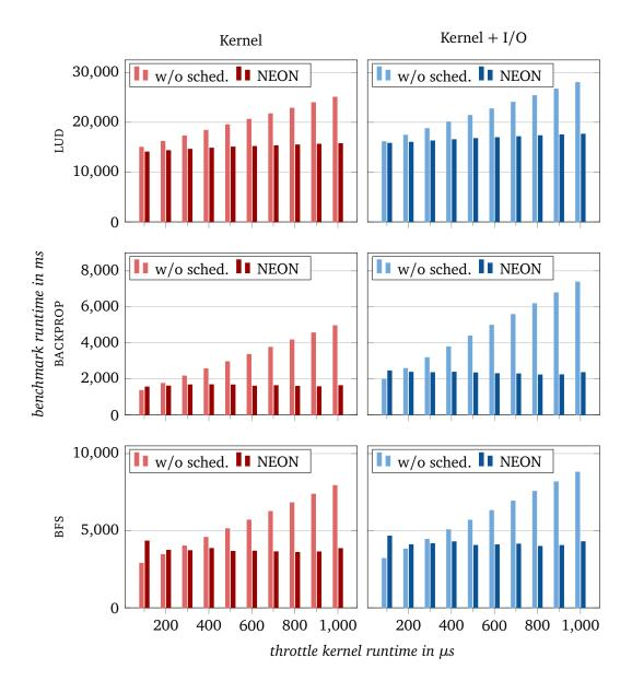
Figure 5.2: Baseline of NEON's scheduling capabilities. Shown are the runtimes of the rodinia benchmarks LUD, BACKPROP, and BFS. Each benchmark runs ten times alongside the throttle application. We configure throttle to create increasing amounts of load. Without any scheduling, throttle occupies increasingly larger shares of GPU time, resulting in longer benchmark runtimes. A perfect scheduler keeps the benchmark runtimes constant, independent of throttle's kernel runtime.
