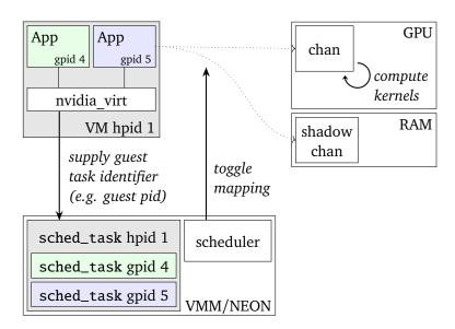
Figure 3.2: Structure of the paravirtual approach: The virtual GPU driver (nvidia\_virt) sends hints during channel creation, that allow the VMM to create separate scheduling data structures (sched\_task) for each task in the virtual machine. The scheduler switches each guest task's channel mapping with a mapping to a *shadow channel* to control GPU access
