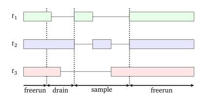
Figure 2.4: NEON's phases. NEON periodically switches between freerun and sampling. Because sampling requires an empty GPU to profile each task, a draining phase is inserted beforehand
