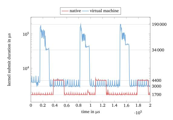
Figure 5.1: Microbenchmark: Durations of kernel submissions on the host and in virtual machines. The plot shows the duration of kernel submissions in an endless loop with a CUDA sync after each iteration. NEON is set to 20 ms sampling and 60 ms freerun. No actual scheduling takes place. A kernel submission during sampling takes approximately 4400  $\mu$ s on the host and 34000  $\mu$ s to 190000  $\mu$ s in the virtual machine with the paravirtual approach.
