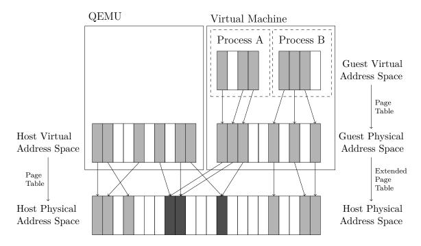
Figure 2.2: The KVM memory setup [20]. Guest virtual addresses are translated to host physical addresses. These translations are managed by KVM using two-dimensional paging if available (as shown), shadow page tables otherwise. QEMU can control the memory of the virtual machine by directing KVM to map the physical memory backing some region of QEMU's virtual address space into the physical address space of the guest ( $\blacksquare$ ).
