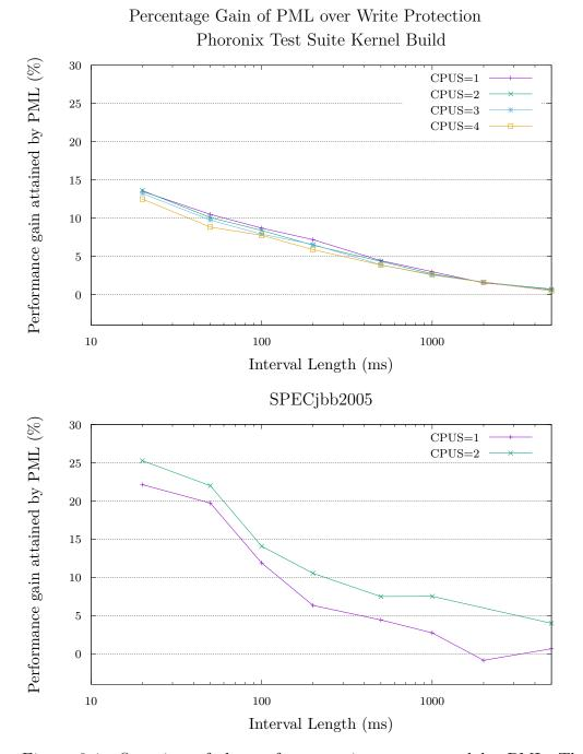
Figure 3.4: Overview of the performance increase created by PML. The horizontal axis denotes interval length on a logarithmic scale, the vertical axis denotes gain of PML over write protection in percent, higher is better. For interval lengths  $\geq 100$ ms, the increase varies between 14% and -1%. At an interval length of 2s and 1, CPU PML causes a decrease in performance, for reasons unkown.
