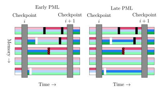
Figure 3.10: Overview of early and late PML activation. When using early activation, write protection is only enabled (■) when it is necessary for COW (■), whereas it is enabled until the next checkpoint or next write access when using late PML activation.
