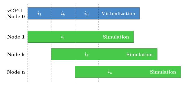
Figure 2.1: Acceleration of full system simulation via SimuBoost. The virtualization node runs the workload and creates checkpoints. Simulation nodes run simulations of intervals, with the respective checkpoint as starting state.
