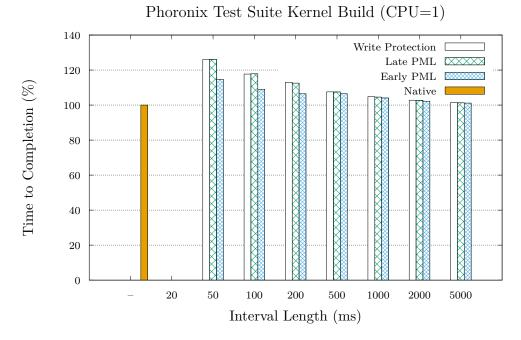
Figure 5.1: The measured time to complete a kernel build for all implementations. Values are in percent of native, lower is better. Write protection and late PML activation are very similar, early activation is able to decrease the run time.
