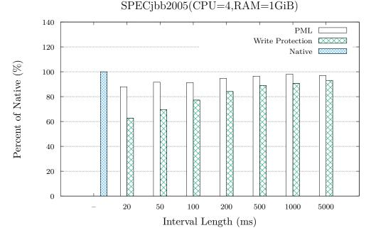
Figure 3.2: Comparison of performance in SPECjbb2005 running with four cores between no dirty logging and dirty logging with PML or write protection. The horizontal axis denotes interval length between polling the dirty bitmap in milliseconds. The vertical axis denotes score in SPECjbb2005, compared to native, higher is better. The results are very similar regardless of the number of CPUs.
