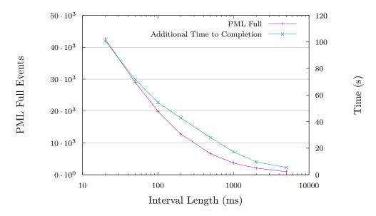
Figure 3.7: Comparison of PML full events introduced by dirty logging via PML compared to the additional time to complete a kernel build. The number of PML full events is given by the left y-axis, the time to completion on the right. Values given are for one CPU. Overall, the curves are similar but not as close as in the same consideration for write protection.
