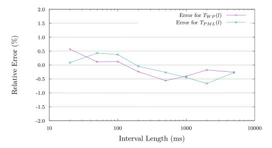
Figure 3.8: The relative errors of  $T_{WP}$  and  $T_{PML}$  to the measured values. Both are accurate to 1%.
