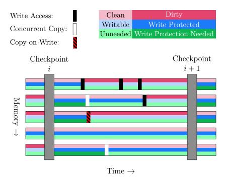
Figure 3.9: Overview of incremental COW checkpointing using write protection for dirty tracking. Write protection is enabled whenever a page is clear.
