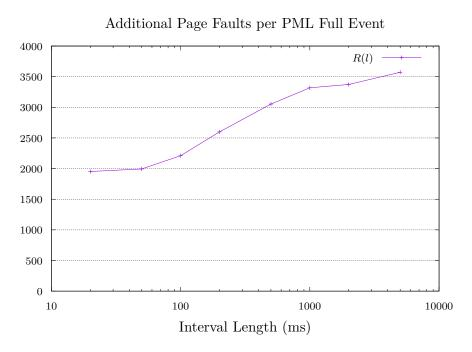
Figure 3.5: The ratio R(l) of additional page faults when performing dirty logging via write protection per introduced PML full event when using PML. The horizontal axis denotes interval length. Values given are for one CPU. The ratio increases with the interval length and can exceed the PML buffer size.
