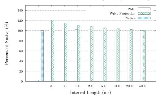
Phoronix Test Suite Kernel Build(CPU=1,RAM=1GiB)
