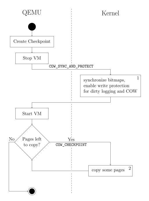
Figure 4.1: Overview of SimuBoosts checkpointing implementation. Elements on the left execute in user space, elements on the right in kernel space. 1 constitutes the work performed during the downtime. 2 is the majority of work, performed asynchronously to workload execution.
