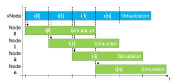
Figure 1: The workload is executed with virtualization. Checkpoints at the interval boundaries serve as starting points for parallel simulations.
