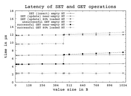
Figure 5.10: Latency for complete SET and GET operations on Falafel between two InfiniBand nodes for an empty, near-empty and an 80% full hash table. The readahead is set to 512 B. The steep increase in latency for get operations around 464 B shows that the readahead is not sufficient from there on.
