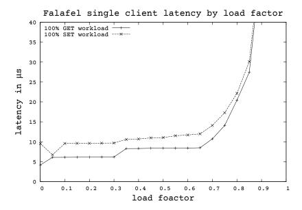
Figure 5.16: Latency for SET and GET workloads depending on the hash table load factor. The measure points are medians of the latencies of 100 000 000 operations.
