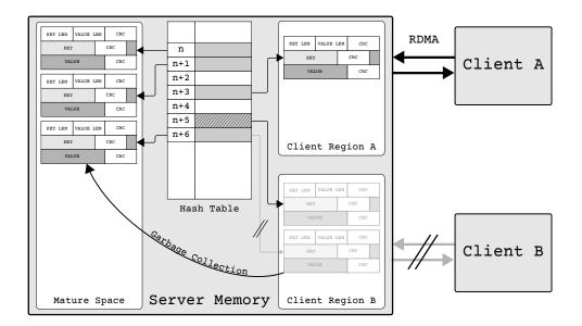
Figure 3.1: Design Overview: server memory with mature space, two client regions and two clients. Client A is connected and may read from the server memory and write to client region A via RDMA. Client B is disconnected. The server garbage collects its client region B, moves the data to the mature space, and updates the hash table entry n + 6. The hash table entry n + 5 is already deleted and will not be preserved.
