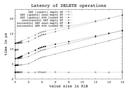
Figure 5.11: Latency for complete SET and GET operations on Falafel between two InfiniBand nodes for value sizes between 8 B and 16 KiB. Between 464 B and 15 KiB the GET latency is higher than the SET latency.
