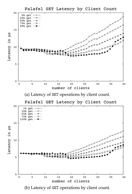
Figure 5.13: SET and GET latency by client count for different workloads. Measure points are medians of 1 000 000 operations. For every workload and client count the hash table load factor is 0.1 We use five client nodes and distribute the clients equally among them. We use a uniform key distribution for SET and GET.
