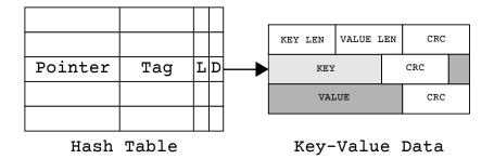
Figure 3.2: A hash table entry with data pointer, tag and Lock/Delete flags pointing to the container with key and value strings.
