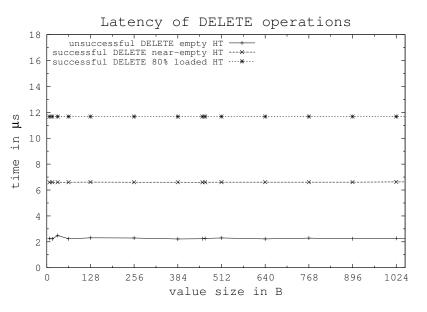
Figure 5.12: Latency for complete DELETE operations on Falafel between two InfiniBand nodes for a near-empty and an 80% full hash table. The readahead is set to 512 B.
