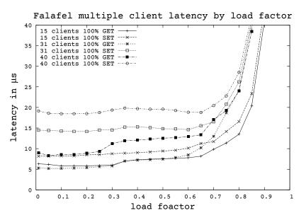
Figure 5.17: Latency for SET and GET workloads depending on the hash table load factor. The measure points are medians of the latencies of 100 000 000 operations.
