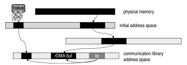
Figure 7. Mapping physically contiguous addresses in native L4 address spaces
