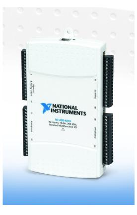
Figure 3.5: NI USB-6218 (picture from http://www.pressebox.de/ pressemeldungen/national-instruments-germany-gmbh/boxid/75241)
