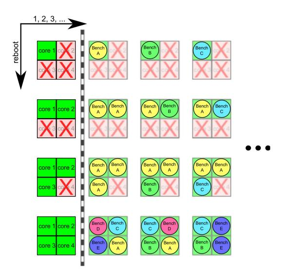
Figure 4.1: Data acquisition by running benchmark permutations
