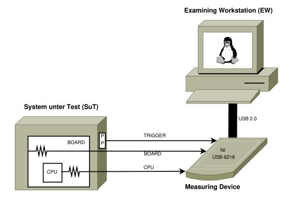
Figure 3.1: Measuring setup overview
