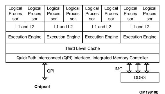
Figure 2.1: Intel<sup>®</sup> Core<sup>TM</sup> i7–2600K Processor cache organization (taken from [12])
