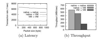
Figure 7: Performance of Torus-Routed Virtualized Networks.
