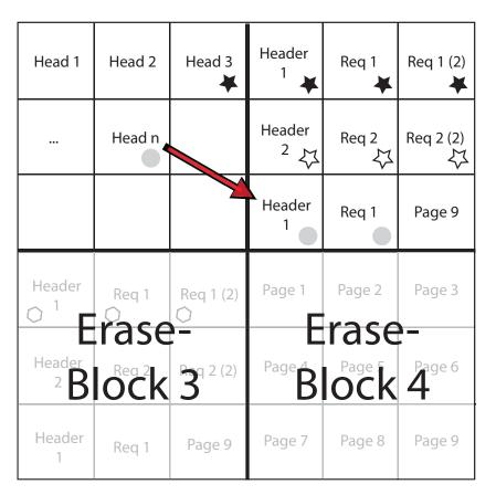
Figure 5.4: The log is optimized for the special characteristics of flash memory. The head-block is zeroed once and then written page per page on a log reset pointing to the start of the log. A special UUID (symbol) allows to differ between valid and old log entries.
