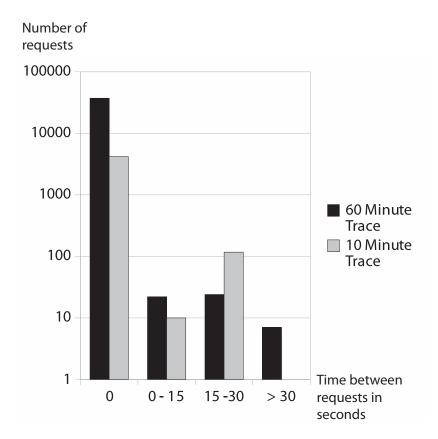
Figure 6.1: The 10 min and 60 min traces show two extremes: While the 10 min trace has no idle times greater than 30s, the 60 min trace has several long idle periods.
