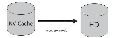
Figure 3.4: In recovery mode the log is replayed from the non-volatile storage to the hard disk.
