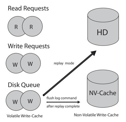
Figure 3.3: While the log is replayed no new read or write requests are processed. Once the replay is complete the log is reset.
