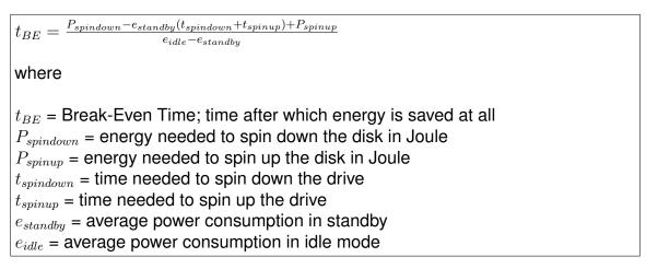
Figure 2.1: Break-Even Time: time after which energy is saved at all
