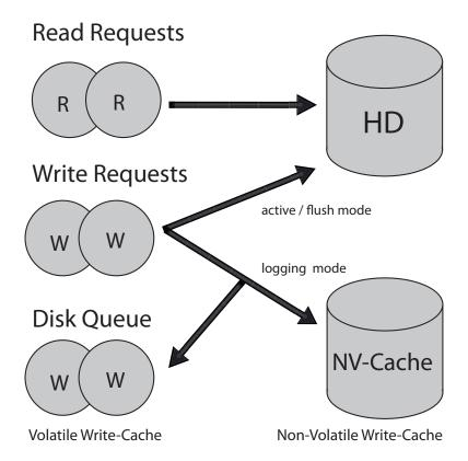
Figure 3.2: Read-Requests are passed through. In active or flush mode Write-Requests are written directly to disk. In logging mode Write-Requests are split and written to a volatile memory queue and a non-volatile cache.
