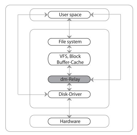
Figure 3.1: The proposed solution is positioned between the buffer cache and the disk driver
