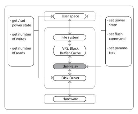
Figure 5.1: The proposed solution is positioned between the buffer cache and the disk driver and an user space interface is provided.
