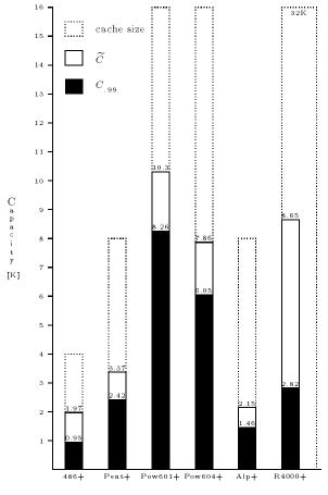
**Figure 5.** Hypothetical Cache Capacities When Adding an 8-overflow Cache
