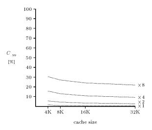
**Figure 1.** Stochastic Capacity, n-way Caches
